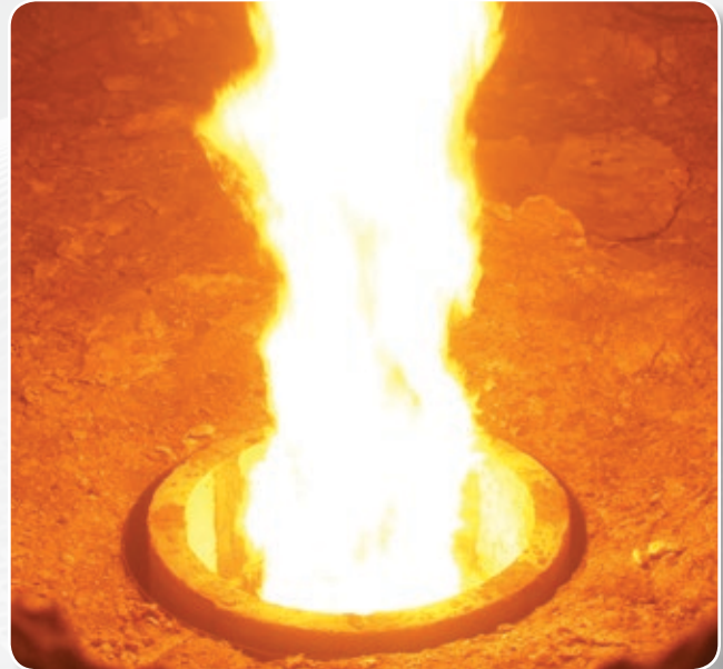
AK Staged Air Low-Emissions Combination Burner Operating on Oil Only
